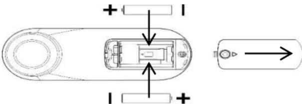
After placing the batteries the AGE Scanner can be turned on:
