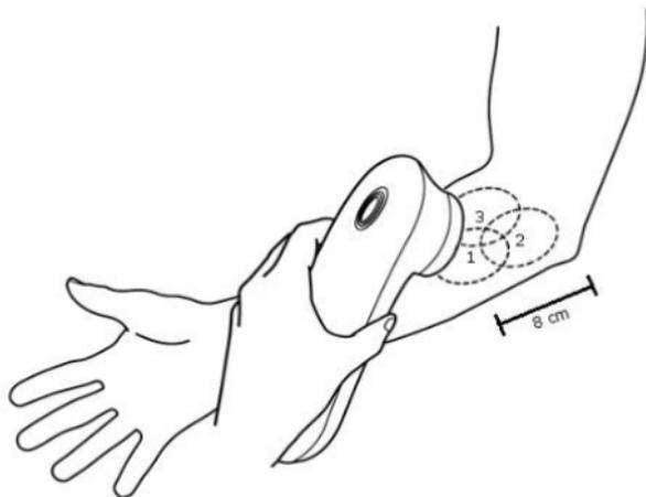
*Measurement location in single mode (fastest result):*
